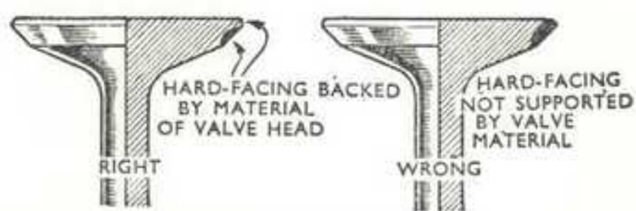
Correct and incorrect techniques in the process of hard-facing valve seat areas.
