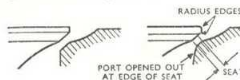
How to reduce the width of the seatings on valve face and inlet port.
