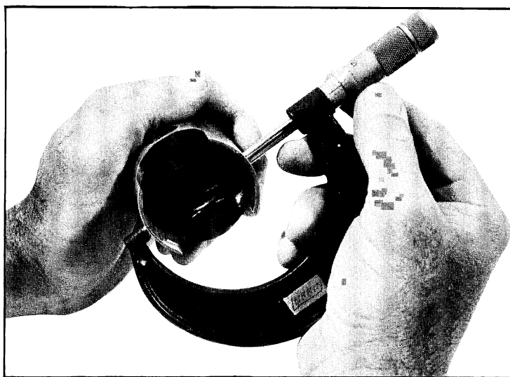
Fig. 11-15 A micrometer is used to measure skirt of piston
