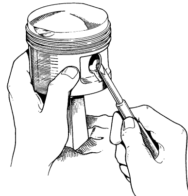
Fig. 11-13 Removing circlip (Triumph Norton Incorporated)
