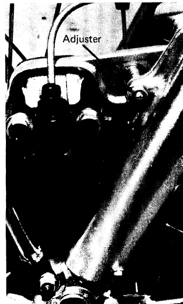
Fig. 6-17 Disc brake threaded caliper adjuster
