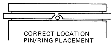
Fig. 9-15 Positioning piston ring; showing correct and incorrect pin-ring relationship
