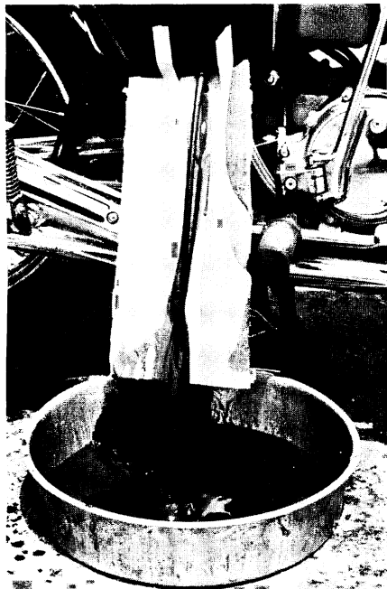
Fig. 14-12 Draining dry sump oil: a cardboard flume can be taped to bike to drain oil away from frame
