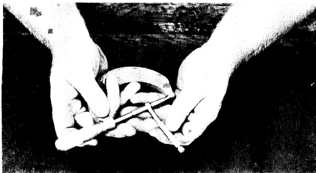
Fig. 7-13 Taking a measurement with a telescoping gauge and micrometer
