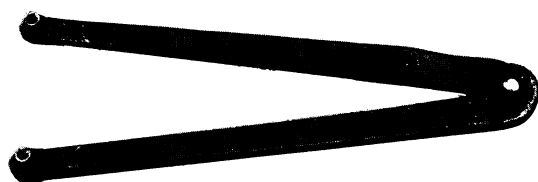
Fig. 3-48 Pin wrench
