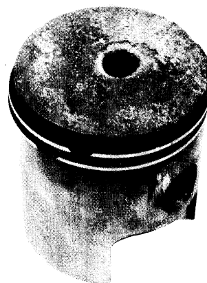
Fig. 8-20 Holed piston showing hole melted in piston during operation with hot plug
