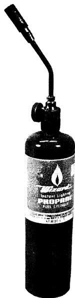
Fig. 3-22 The propane torch is used for metal bending and soldering.
