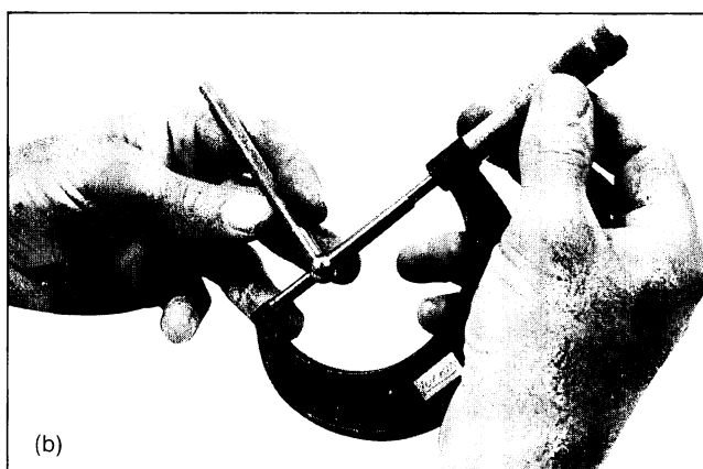
Fig. 9-11 Measuring the cylinder bore, showing (a) snap gauge in cylinder bore and (b) micrometer on snap gauge
