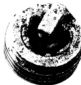
Fig. 21-35 Oil-fouled plug (AC Spark Plug Division of General Motors Corporation)
