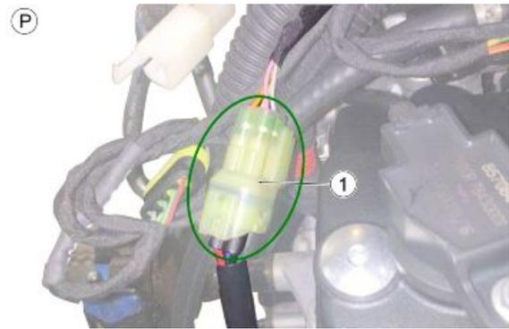
**TABLE P1 - POSITIONING AND CONNECTING THE STAND SWITCH**
