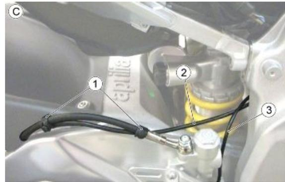
**TABLE C1 - REAR SWINGARM ZONE AND REAR STOP AND ABS SENSOR CABLE ROUTE ON CHASSIS**
