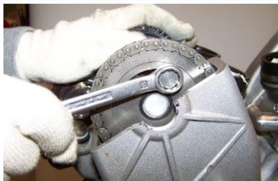
**Specific tooling****020850Y Primary gear lock****020914Y Flywheel stop**
