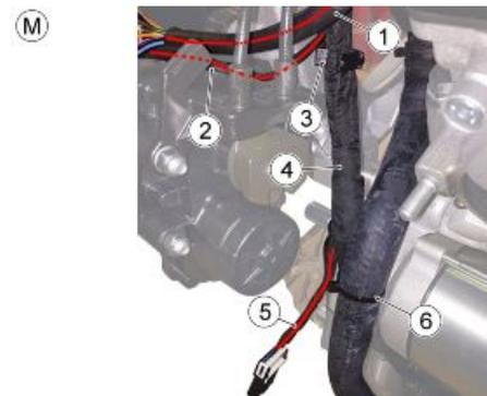
**TABLE M1 - CABLE ROUTING EXHAUST VALVE MOTOR ZONE**
