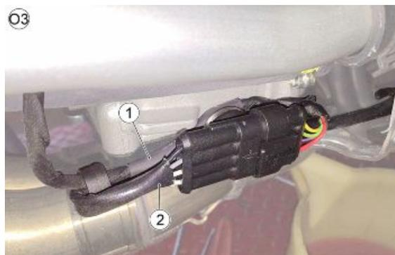
**TABLE P - POSITIONING AND CONNECTING THE STAND SWITCH**
