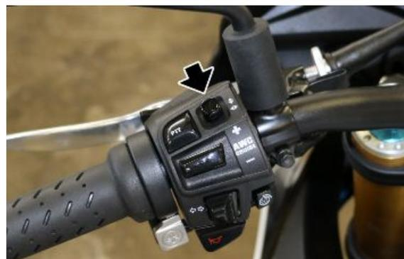
This function allows you to disable the ABS system that is normally active "On".
