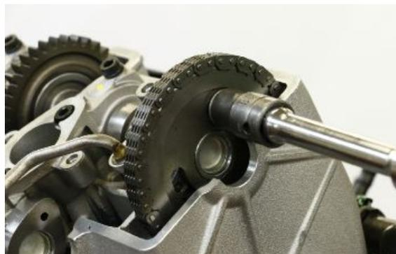
screw. This screw must be replaced at each reassembly.
