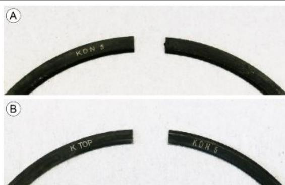
The five ring gaps (two piston rings, two oil scraper rings, one oil scraper spring) are fitted displaced 90° to each other, starting from the exhaust-side stud bolt opposite the chain and continuing clockwise.
