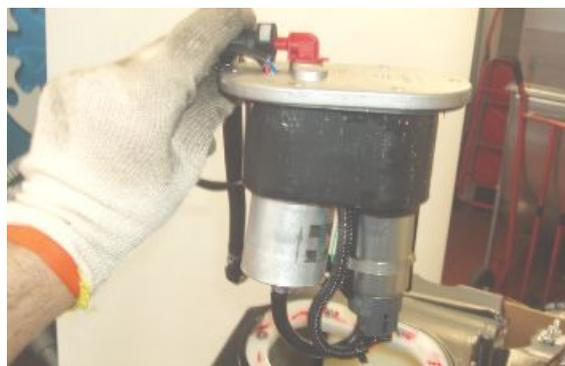
PIN 1-2: 0.5 - 1 ohm; PIN 3-4: you do not need to measure the component electrical resistance since it works correctly with suitable supply from the instrument panel only. Check correct operation as follows: connect in series a bulb of approximately 2 W: it should turn on if the tank is in reserve, otherwise, it remains off.
