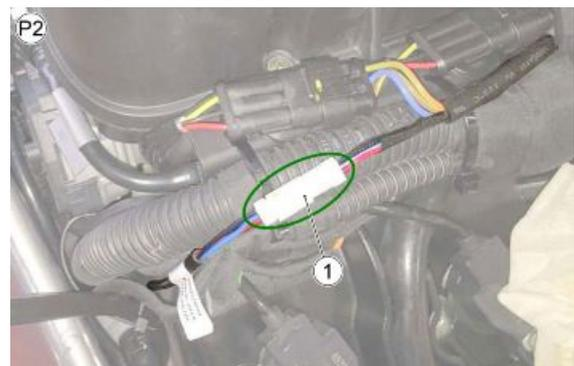
**TABLE P3 - POSITIONING AND CONNECTING THE STAND SWITCH**
