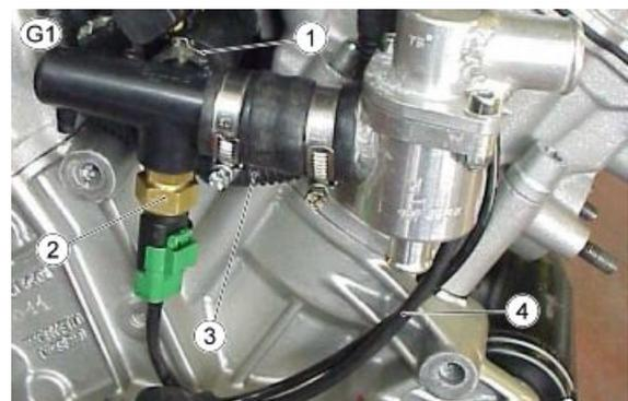
**TABLE G2 - WATER TEMPERATURE SENSOR AND INJECTORS CONNECTION**
