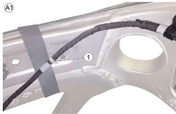
**TABLE A2 - VEHICLE WIRING HARNESS ON CHASSIS**
