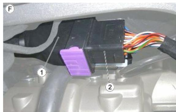
**TABLE F1 - INTERCONNECTION BETWEEN ENGINE WIRING HARNESS AND MAIN WIRING HARNESS**
