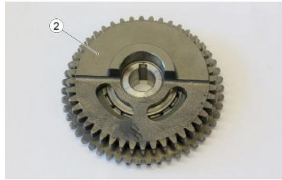
If deformations or broken material are found on the sliding surface, replace the freewheel gear (2).
