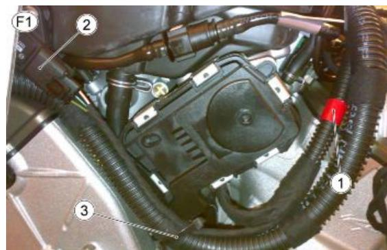
**TABLE G - WATER TEMPERATURE SENSOR AND INJECTORS CONNECTION**
