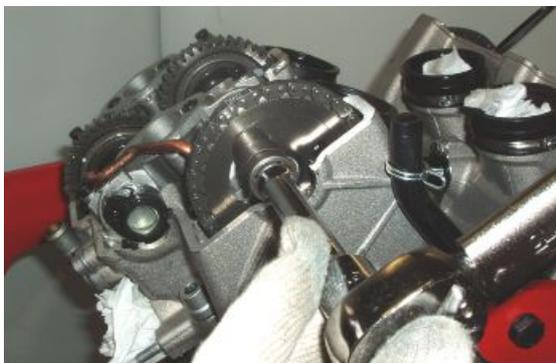
**Specific tooling****020851Y Camshaft timing pin****020852Y Crankshaft timing pin**
