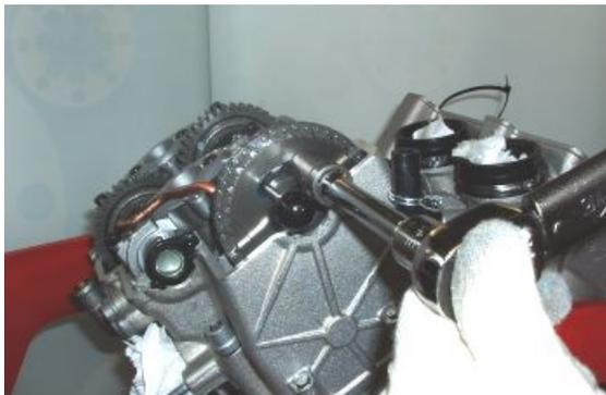
**Specific tooling****020850Y Primary gear lock****020914Y Flywheel stop**
